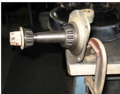
Using the same spindle and clamp with a front hub (no drum attached), and clamped onto a piece of pipe, this makes the perfect tool for spray painting wheel rims.
