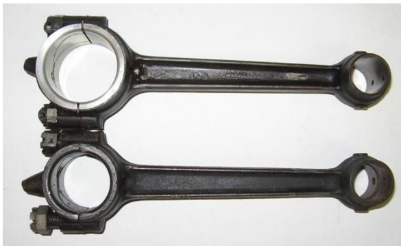
Comparison of 1932 Model B (top) rod to Model A Rod, they are the same length with a 1" piston pin. Journals: A = 1-1/2" B = 1/7/8"
