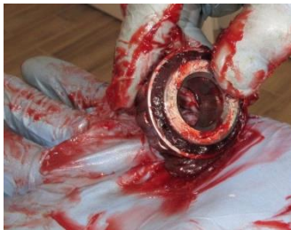
Completely pack the bearing with grease (NLGI-2 rated)
