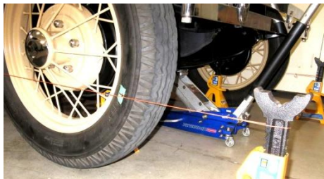
Front string intersect and jack stands
